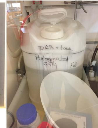
C. Separation of halogenated vs. non halogenated solvents
