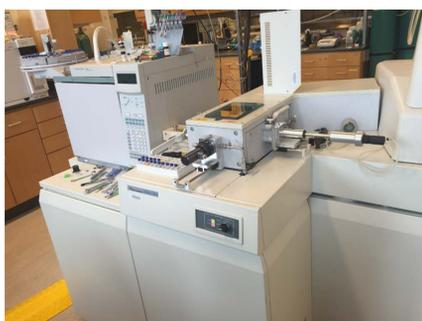
Fig. 1. Example instrument in our lab: Pyroprobe autosampler, GC-MS in Summons Geobiology Laboratory, Massachusetts Institute of Technology.
